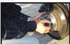
Mount the wheel spacer on the axle using the nuts/bolts which were included in the delivery. Tighten the nuts/bolts by hand.
