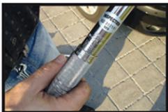
Using a torque wrench. Tighten to the vehicle manufacturers-specifications.
