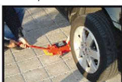
Raise the vehicle enough to remove the axle stands, then slowly lower the lifting jack.
